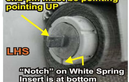
Re-insert the end-bracket and re-fasten end-bracket screws. We recommend you fasten them only part way first so you may test the tension of the unit. If tension is adequate, fasten them fully, if tension is not adequate, repeat steps 2 and (the first part) of 3 until the desired tension has been achieved.
